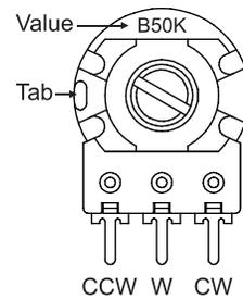
There is a tab on the pots that must be removed or it will get in the way when you try to mount them in the enclosure or panel. Hold the pot in one hand and grab the tab with a small pair of pliers. Rotate the pliers away from the pot, and the tab will snap right off.
